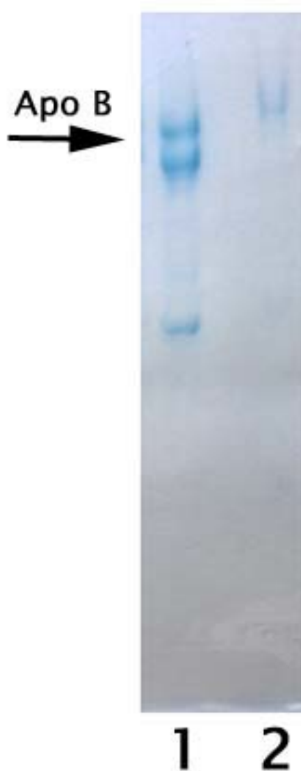
Figure 2: SDS PAGE Gels of Purified Lipoproteins. 20 \mu\text{g} of LDL/VLDL purified by the STA-608 kit (lane 1) or ultracentrifugation (lane 2) was loaded on a 3-8% Tris Acetate Gel (A) or a 12% Bis Tris Gel (B) and stained with Coomassie Brilliant Blue Dye.
