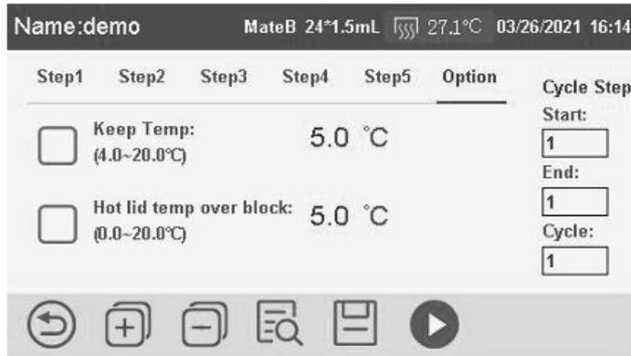
**Keep temp.:** Block will maintain the setting temperature after all steps finished, default is 5.0°C. The function open after tick the box.
