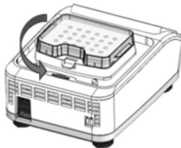
e) Pull up the eccentric wheel handle to a vertical position.
