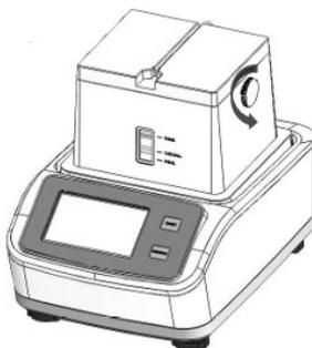
Attentions: Please ensure the heating plate of hot lid do not touch with block when the instrument mixing function is on.
